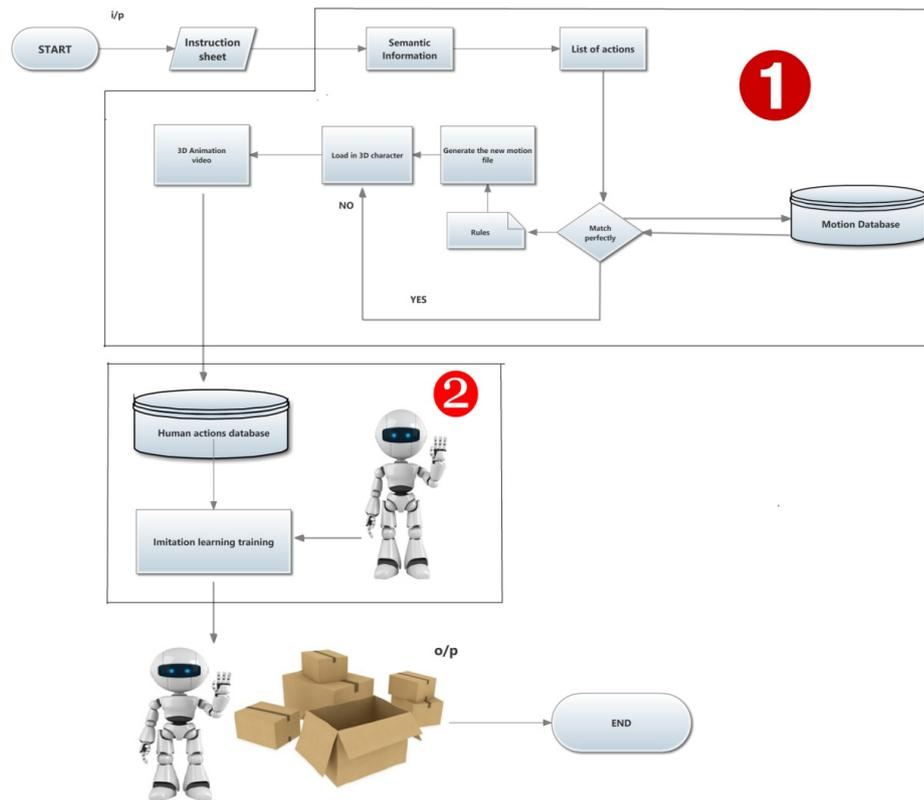
**Fig. 5.** Automatic packaging simulation pipeline
